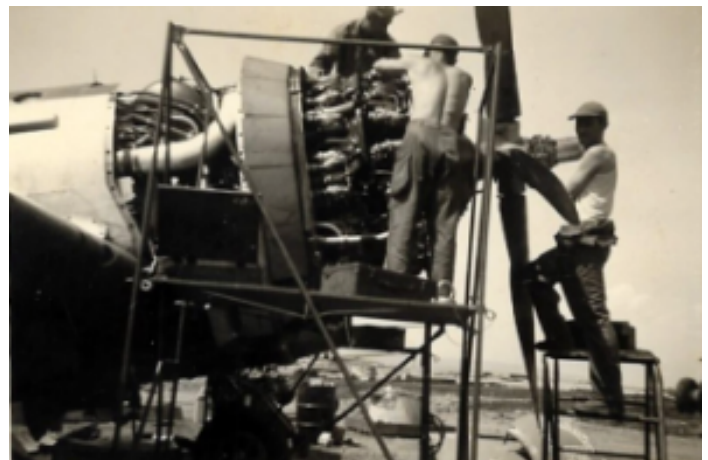
Engine change or engine maintenance of a P-47 of the 394th FS. Note the 2 rows of cylinders (Linda Tjepkes/archives 367 th FG)
