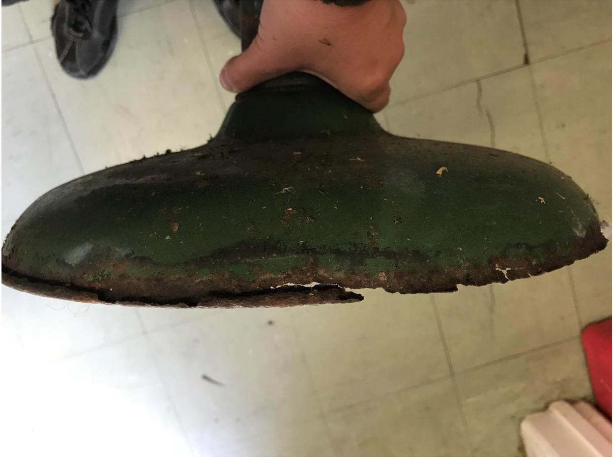
The dark green gloss paint is mostly in good condition after 60+ years in the undergrowth. The electric shroud fitting is corroded, and the white inside and edge is stained with some rust but, given that it has spent the interim in the open, it is in remarkable condition. They were used everywhere, from offices to radio sites; parachute packing blocks to latrines.
