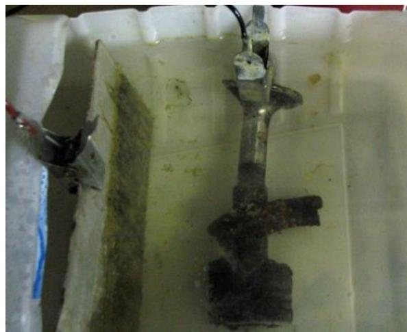
Far left, a valve of one of the engine of the P-38J-10-LO 42-67909. Left, the same valve being cleaned by electrolysis
